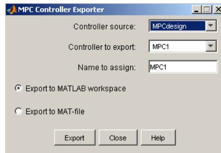
Figure 4-13: Exporting a Controller to the Workspace
